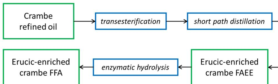
Figure 3: process roadmap to obtain the deliverable samples of oils concentrated in erucic acid using crambe refined oil as starting material.
