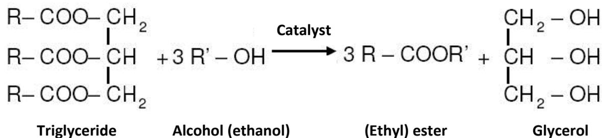
Figure 1: general transesterification reaction. In parenthesis, specific case of obtaining ethyl esters.
