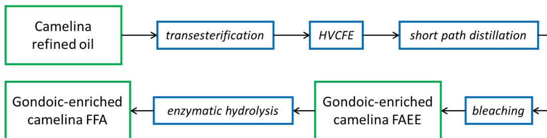
Figure 2: process roadmap to obtain the deliverable samples of oil concentrated in gondoic acid using as starting material camelina refined oil.
